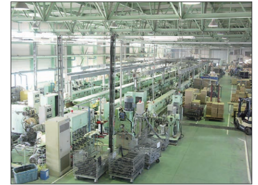
連続加硫ライン Continuous vulcanizing lines
