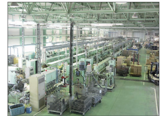
連続加硫ライン Continuous vulcanizing lines
