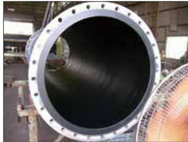
接着剤塗布 / After Adhesive Coating
