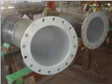
下地処理 / After Pre-Treatment
