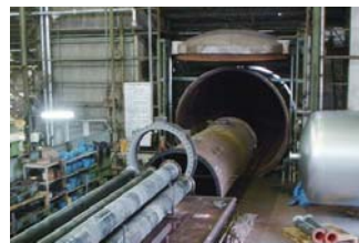
大型加硫缶 Large-Sized Vulcanizing Autoclave (4,000φ×15,000L)
