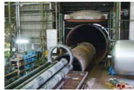
大型加硫缶 Large-Sized Vulcanizing Autoclave (4,000φ×15,000L)
