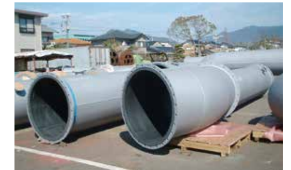
排煙脱硫装置配管 Pipes for Flue Gas Desulfurization Plant
