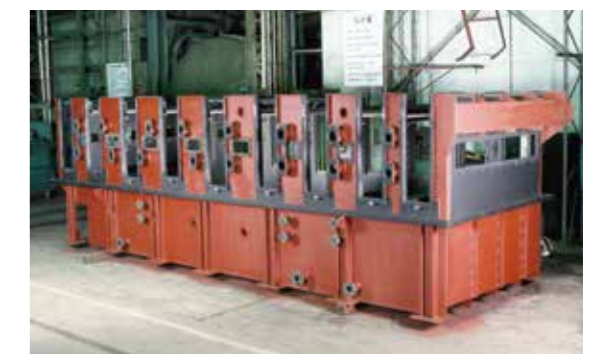
精錬工場向け酸洗槽 Pickling Tank for Iron & Steel Plant
